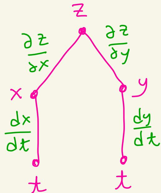
$$\frac{dz}{dt} = \frac{\partial z}{\partial x} \frac{dx}{dt} + \frac{\partial z}{\partial y} \frac{dy}{dt}$$
